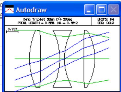
8. Adjust the radius of surface 6 to restore the focal length to 10 mm using the following method:
