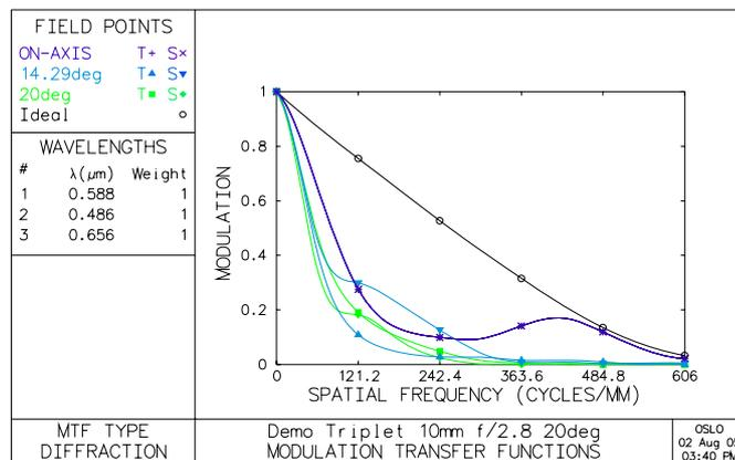
27. From the **Evaluate** menu header select **Transfer function** ► **Through frequency report graphic ...** and enter the figure calculated (**606.0**) in the box labelled **Maximum frequency**.
