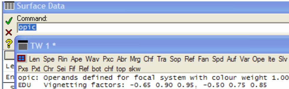
Note the message in the text window. The “Vignetting factors” on the second line are the (relative) values of **ymin**, **ymax** and **xmax** for the two off-axis points, at (relative) field heights of 0.7 and 1.0 respectively. These figures will be used to set the rays drawn in the lens drawing conditions spreadsheet (see below).
