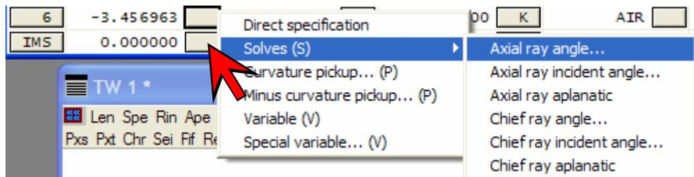
Right-click on the grey RADIUS button for surface number 6, and select **Solves(S)** ▶ **Axial ray angle ...** ▶ **Enter solve value: -0.1785714** (note that this is -0.1 times the entrance beam radius)
