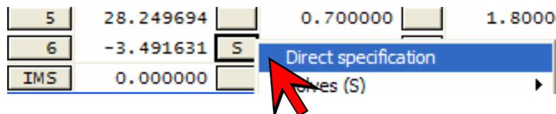
9. Remove the curvature solve on surface 6: Click on the grey RADIUS button for surface 6, and select **Direct specification**. The “S” should vanish.
